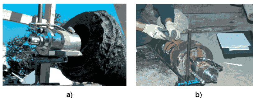
Figure 3. Radiographic recording a) barrel of the French ship cannon, AN 1808 RUEELLE, b) barrel of the French cannon 75/27 model 1911 Deport (Military Museum in Kalemegdan in Belgrade)
