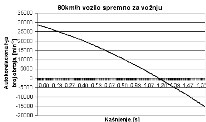
Slika 17 – Autokorelaciona funkcija broja obrtaja Picture 17 – Autocorrelation function of number of wheel's speed
