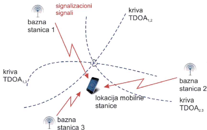
Slika 3 – Određivanje lokacije MS u presečištu tri hiperbole Figure 3 – Determination of the MS location at the intersection of three hyperbolas
